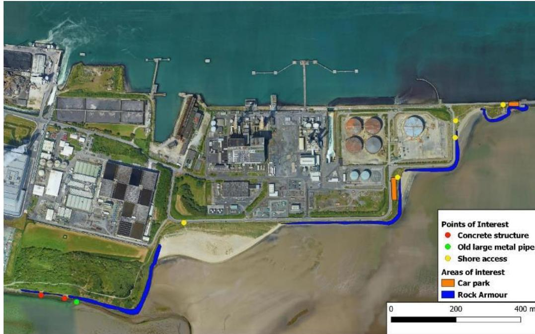
Figure 3.40: Location of Rock armour in the Poolbeg survey area.
